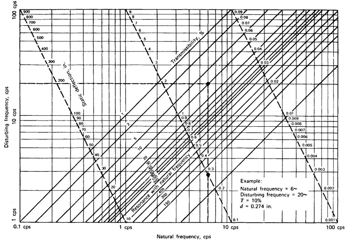
Fig. 24.4 Transmissibility of flexible mountings:  $T = 1/[(\omega/\omega)^2 - 1]$ .
