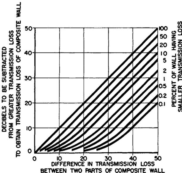
**Fig. 24.3** Decibels to be subtracted from greater transmission loss to obtain transmission loss of composite wall. The difference in transmission loss between two parts of composite wall. Percentage of wall having smaller transmission loss.
